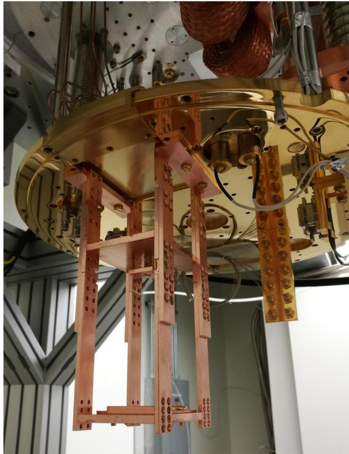
Copper cage mounted rigidly to 3 K plate of Bluefors fridge
